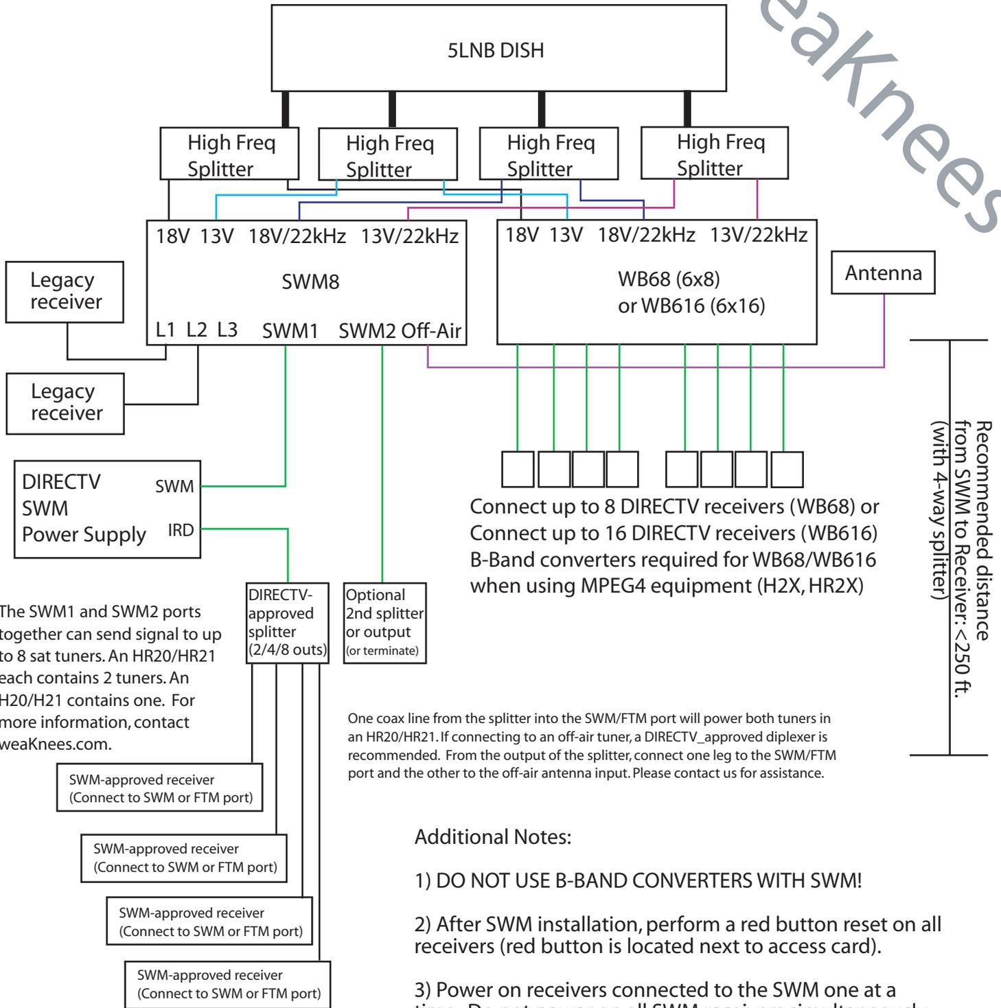
In the diagram above, if each of the four SWM-approved receivers is a DVR, then the SWM2 port must be terminated, as all 8 tuners will be used. On the other hand, if all four are basic non-DVRs (eg. H20/H21), then four additional sat tuners can be connected to either the SWM1 or SWM2 port. For more information, contact weaKnees.com.
